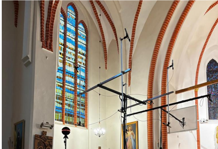
Figure 1: 3D microphone array during recording
